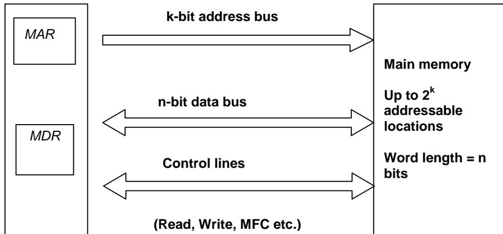
**Figure 9.4: Connection of main memory to CPU**
