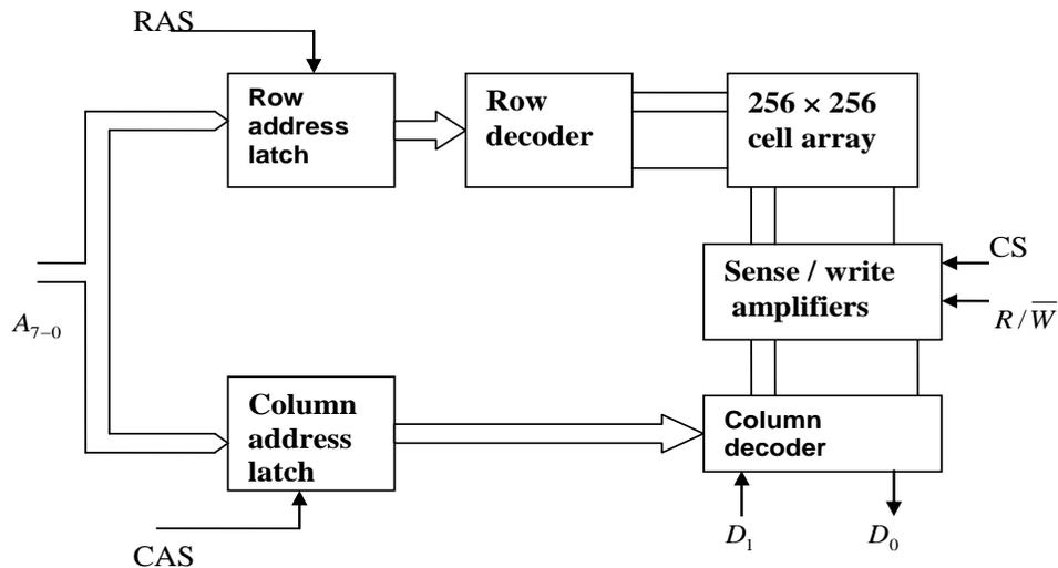
**Fig. 9.7: Internal organization of a 64K × 1 dynamic memory chip**
