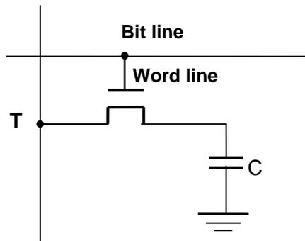
**Fig. 9.6: A single-transistor dynamic memory cell**
