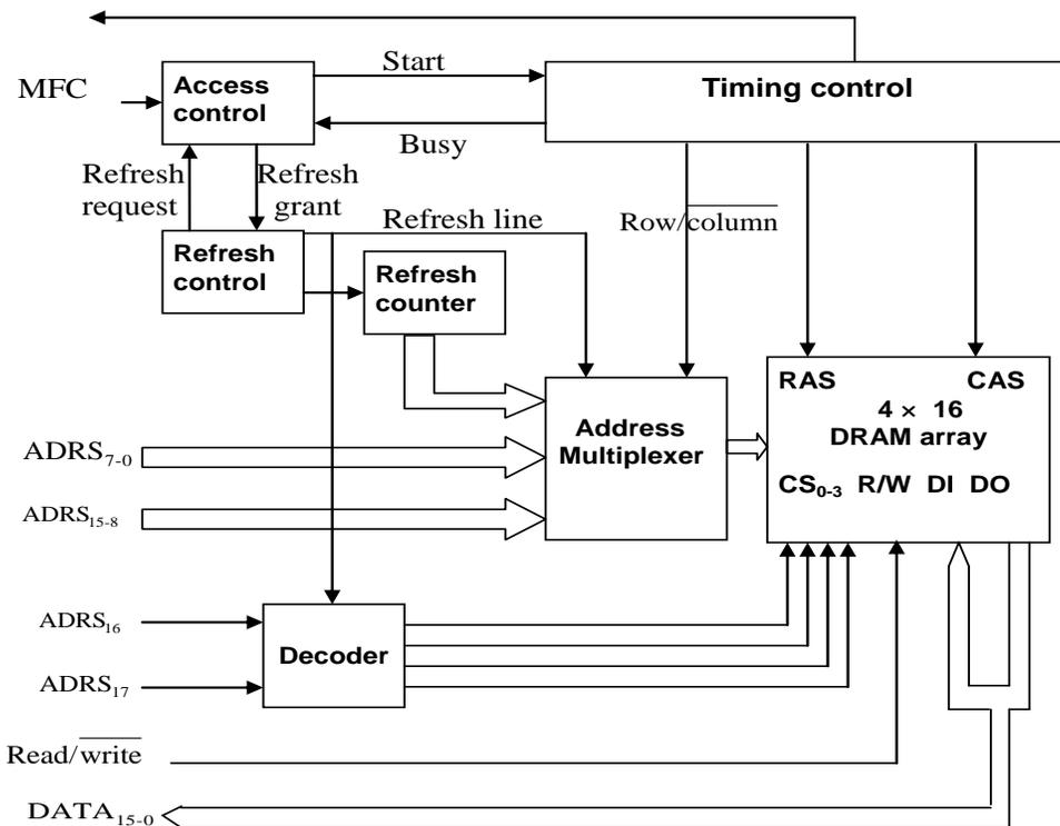
**Figure 9.9: A block diagram of a  $256 \times 16$  dynamic memory chip**
