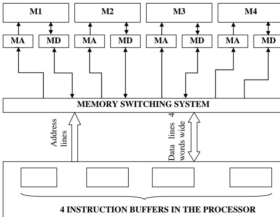
Figure 9.10: Memory interleaving
