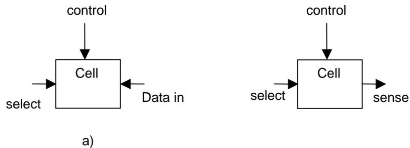
Figure 9.1: Memory cell organization (a) : write (b) for read operation
