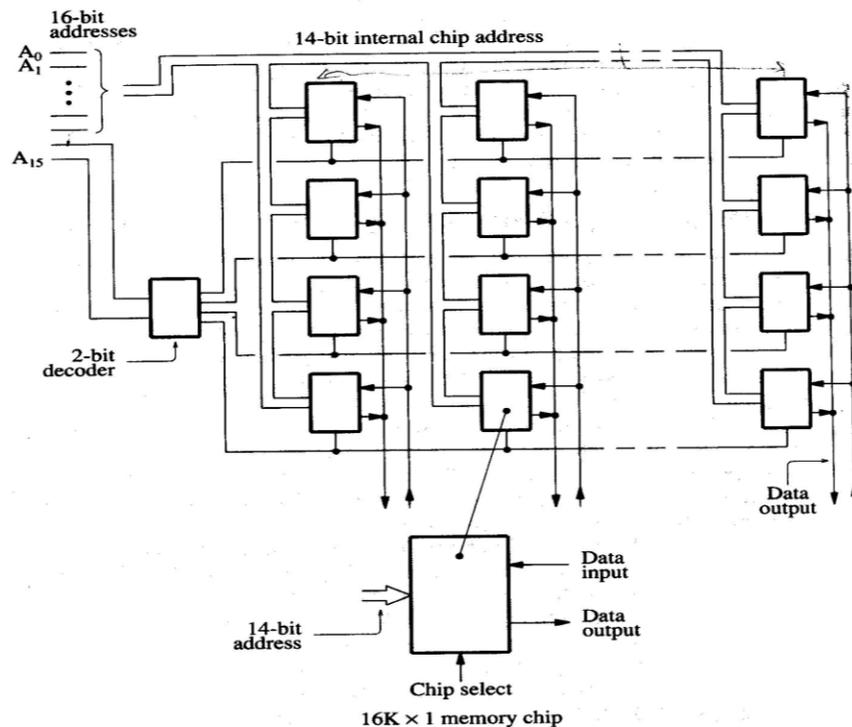
**Fig. 9.8: Organization of a  $64K \times 16$  memory using static memory chips**
