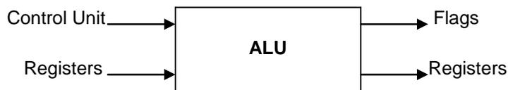
**Figure 7.1: ALU Inputs and Outputs**
