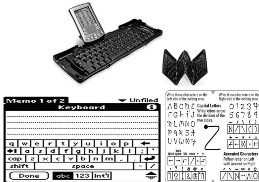
Fig. 12.1: Keyboard and keypads for small devices
